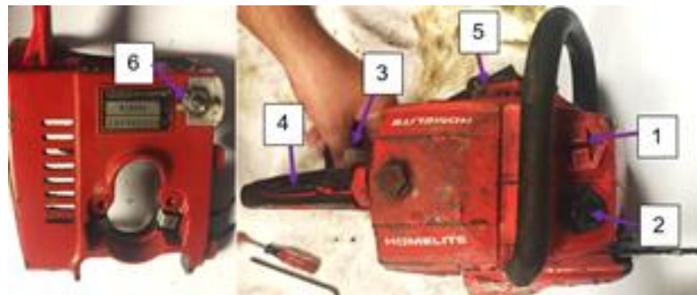
Figure 2: Back Panel view and Top view of Chainsaw: (1) Fuel, (2) Lubricant, (3) Choke, (4) Throttle, (5) Starter Cord, (6) Kill Switch
