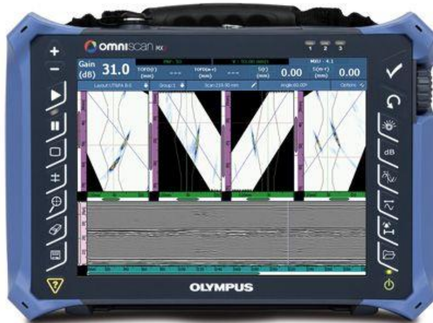
Figure XII-XII.C.2: LSU's Phased Array Ultrasonic Testing [20]
